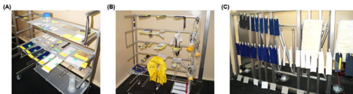
FIG 3 Material samples after 10 dry fogging cycles. (A and B) Various material samples from the aircraft cabin. (C) Fabric, leather, and paint samples.
