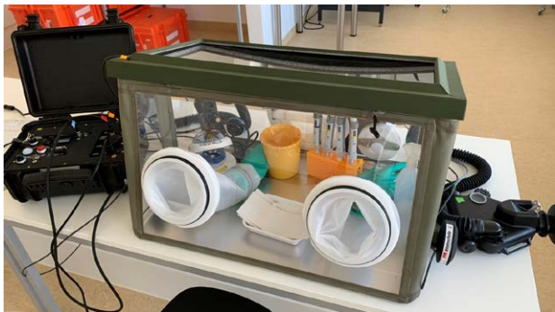
Glove box with technical control unit (left) and blower unit (right side). Photo: S. Weiß
